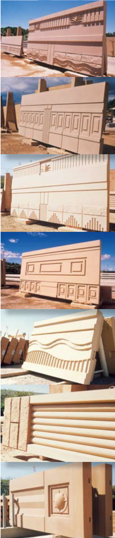
The Nimitz-MacArthur Pacific Command Headquarters in Oahu, Hawaii, used seven types of form liners to create unique patterns in the architectural precast concrete panels used to clad the structure. Photos: Gary Hofheimer Photography.
